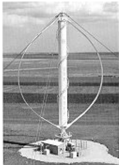
Fig. 4 Vertical-axis turbine (Darrieus design)
