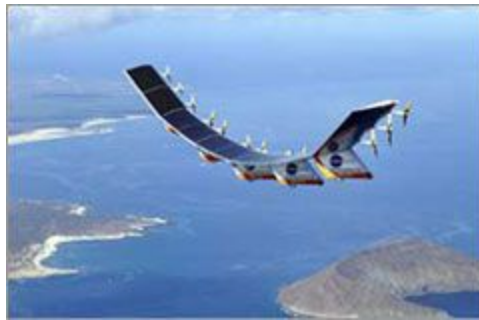
The Helios prototype flying wing is shown near the Hawaiian Islands during its first test flight on solar power. (Credit: NASA, Dryden Flight Research Center Photo Collection)
